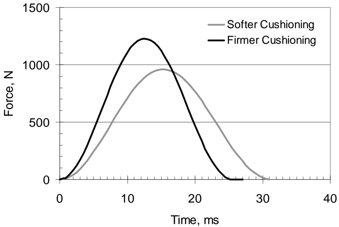
Figure 2: Effect of cushioning on force-time during impact.
